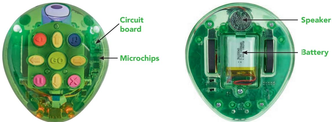
There is one external connector on the back of E.a.R.L. This is used to charge E.a.R.L. The link between charging the robot (E.a.R.L.) and the battery holding that charge could be made. Children should develop an understanding that electrical power is needed by computing devices e.g. mobile phones, tablet computers etc. (Also see the 'label E.a.R.L.' activity sheet at the end of this document).
