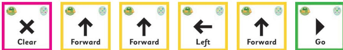
The sequence could be recorded horizontally or vertically. Also note the idea of using "Clear" at the start of the sequence and "Go" at the end. Using "Clear" at the beginning introduces the programming concept of initialisation i.e. things that have to happen before the main program is executed.
